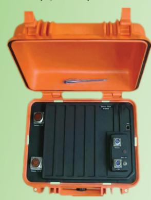
The "Diogen-24/24" can be applied as one of seismic modules of system and it's successfully used for refraction or reflection, downhole or VSP, earthquake monitoring.
